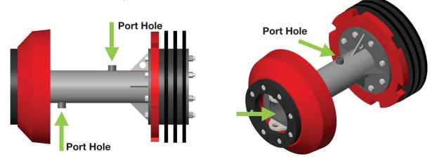
Inhibitor travels through the hollow front mandrel and two port holes located on either side of the mandrel, ultimately leaving a film of protective corrosion inhibitor on the pipe wall.
