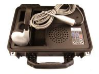
The CDI GeoEAR is very simple to use. It works by amplifying the sounds produced by pigs moving through pipelines and presenting them to a listener through either the headphones, built-in speaker, or both simultaneously.
