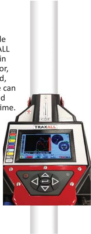
When TRAXALL is aligned with the pipeline as shown here, the pipe legend decal will match the Y axis (green) plot, the X axis (red) plot will represent magnitude perpendicular to the pipeline, and the Z axis (blue) will represent an up/down measurement.
