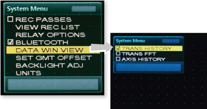
TRANS HISTORY is the default data display mode. It is an X-Y graph, where X=Time and Y=Signal Magnitude. When TRAXALL is set to TRANS HISTORY, passage data can be viewed in real time, or, if recorded, the log file can be replayed at a later time.
