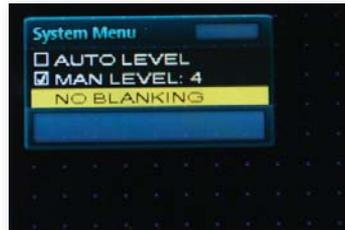
\* ALS levels are 1 through 4. Level 5 is accessible only in manual mode and should be used only when necessary (i.e., when working under bright sunlight) as it can draw extra battery current.
