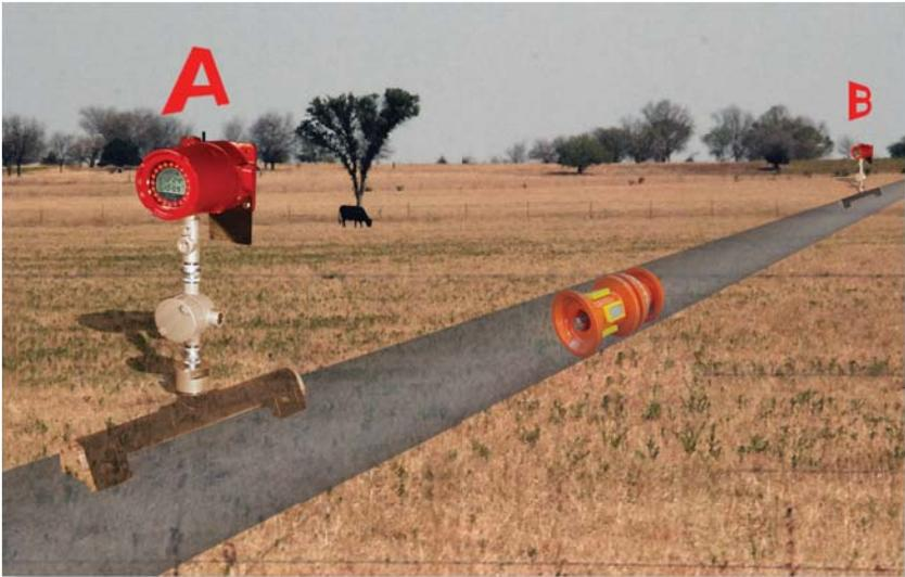
\*MFL pigs are not located with the Pinpointer; rather, you use the tracking capability to locate the magnetic passage detection (see Tracking Example 2, pg. 27)
