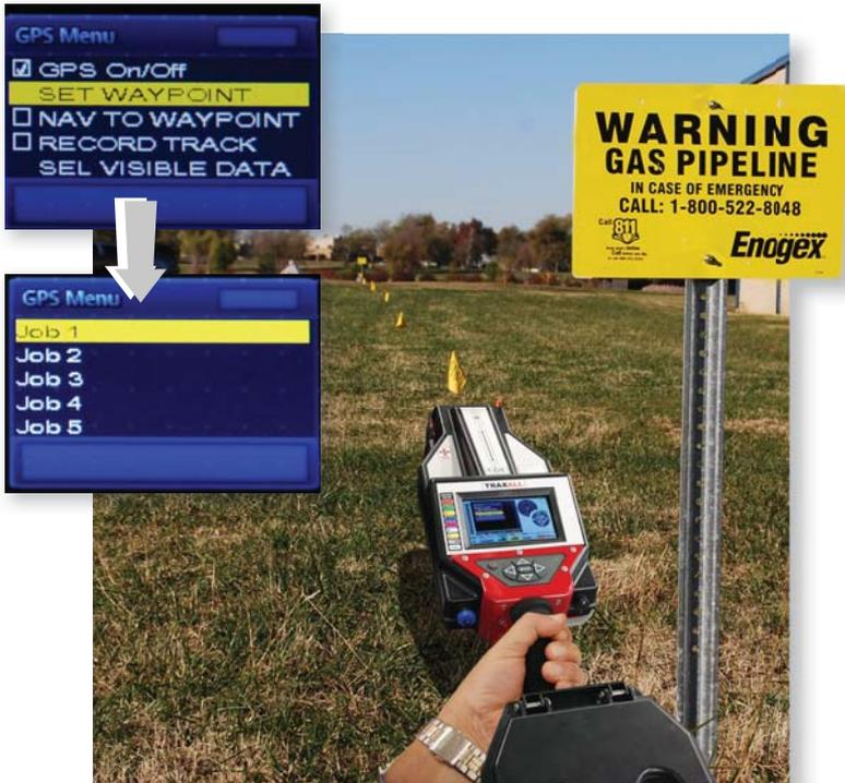
When the TRAXALL receiver is positioned at the desired waypoint:
