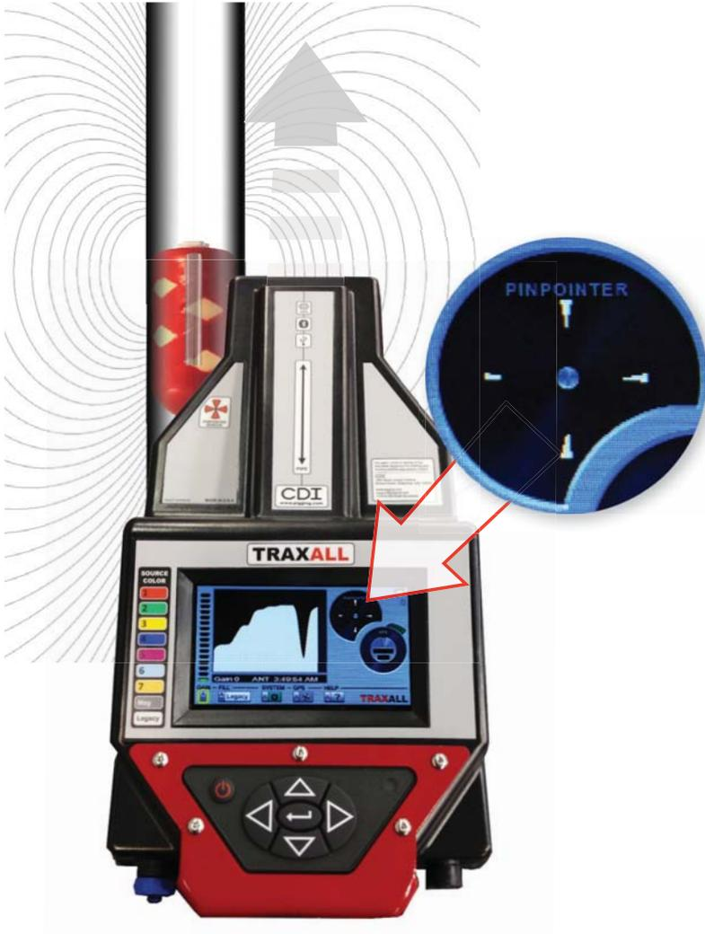
Note dip in History Window graph, and diminished pinpointer markers. Both indicate that the TRAXALL is over the magnetic “null” zone of a legacy transmitter.
