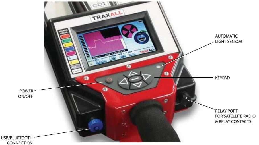
Depress button for 3–5 seconds to power up the TRAXALL receiver (same to power down).
