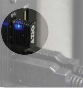
If your PC or laptop does not have built-in Bluetooth, insert a Bluetooth adapter (“dongle”) into its USB port as shown here.
