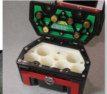
Close the compartment. Make sure screws are firmly seated to maintain a weatherproof seal.
