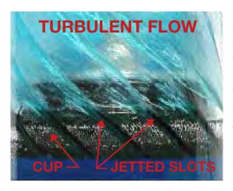
The design of the jetting grooves on the lip of the cup promote the pig to rotate as it travels, ensuring even wear of the cup. This increases cup life and reduces operating costs.
