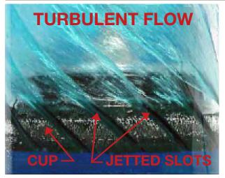
The design of the jetting grooves on the lip of the cup promote the pig to rotate as it travels, ensuring even wear of the cup. This increases cup life and reduces operating costs.
