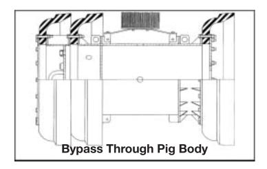
This bypass also lets the pig slip slightly in the stream so that the wax that has been removed can be floated away in the faster flowing stream in front of the pig rather than be pushed into a solid mass. This will also avoid the potentially serious problems which could occur if the wax arrives as a solid plug at the receiving trap.
