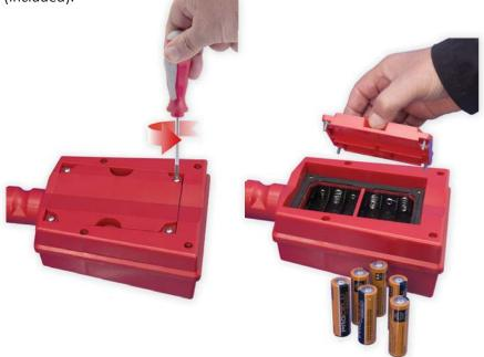
Insert six AA-cell alkaline batteries (also included). Observe battery polarity as shown on receptacle. Check seal for deformation, cracks, tears, or foreign objects. Replace cover.
