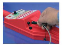
The TRAXALL internal antenna is automatically bypassed when the remote antenna's easily-attached 20 ft [6 m] cable is connected.
