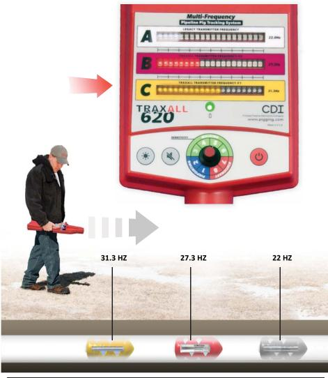
Whether detecting a passage, tracking, or locating, you are looking for the maximum (peak) wave of a transmitter signal.
