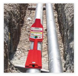
The TRAXALL can be positioned at a Pig Trap to confirm arrival or behind a valve to confirm clearance.
