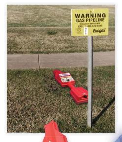
The TRAXALL may be positioned directly onto an exposed pipeline. (Note molded shape on case bottom to aid alignment.)
