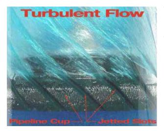
The turbulence created, jets away debris from in front of the cleaning pig. The grooves in the surface of the cup allow a calibrated amount of fluid to pass along the wall of the pipe to jet away wax, sand and other debris.
