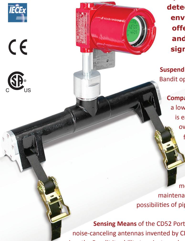
**FOR OVER TEN YEARS, THE CD52 BANDIT has meant simple, reliable, and durable pipeline pig passage detection in the world's most demanding environments. Now, the CD52 Portable Bandit offers the added flexibility of quick takedown and relocation wherever/whenever a temporary signaler is needed.**
