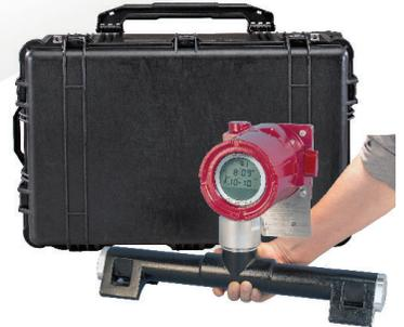
**Sensing Means** of the CD52 Portable Bandit consist of a set of patented, non-intrusive proprietary noise-canceling antennas invented by CDI specifically for pig passage detection. This antenna system gives the Bandit its ability to reject nearby magnetic noise and halt costly false-positive triggering. A small, safe, permanent magnet or active transmitter installed on a pig is all it takes to put the Bandit to work!
