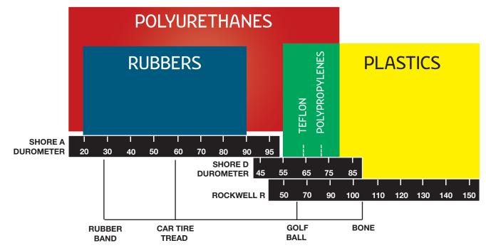
In regards to pipeline pigs, each Durometer has its advantages and disadvantages. The description headings below also indicates our standard color for each Durometer:
