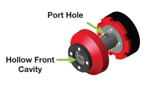
Inhibitor travels through the hollow front mandrel and two port holes located on either side of the mandrel, ultimately leaving a film of protective corrosion inhibitor on the pipe wall.
